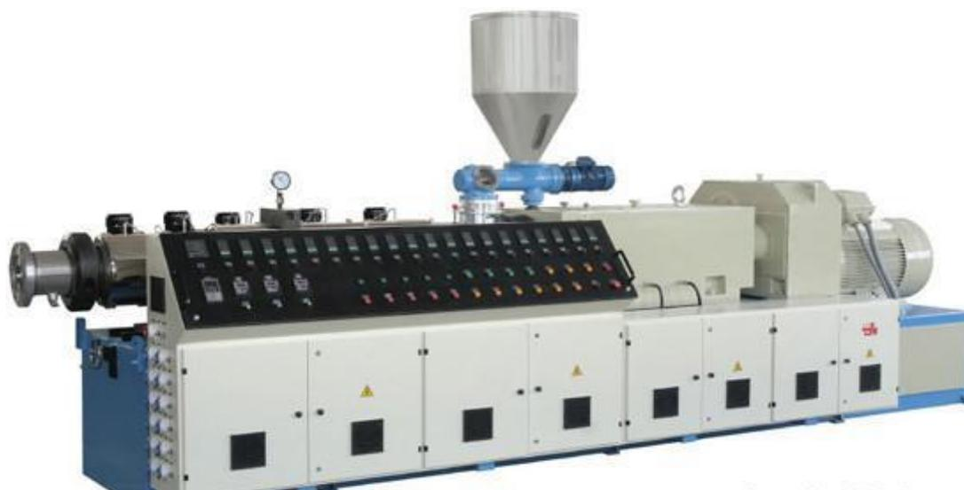
Figure 2: Single Screw Extruder
