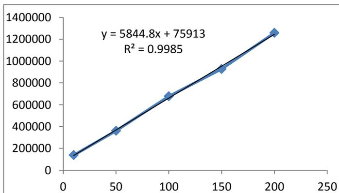
**Figure 3: Calibration curve of olopatadine by RP –HPLC method**
