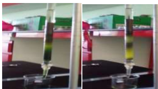
Figure 3: Fractionation process of Morindacitifolia leaves extract
