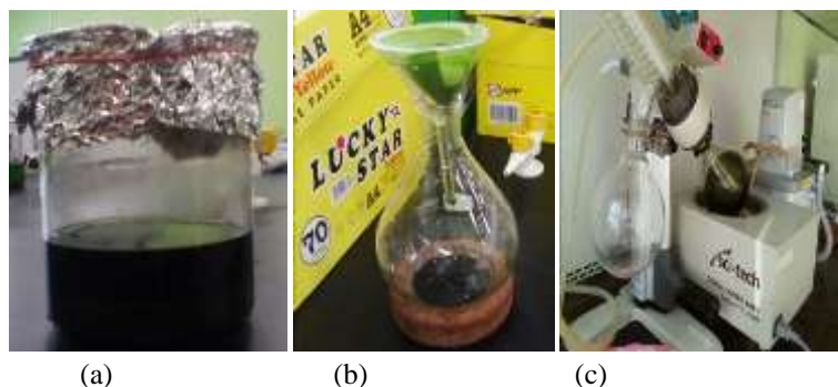
Figure 2: (a) Maceration of the leaves, (b) Filtration process, and (c) Drying process of the filtrate using rotary evaporator
