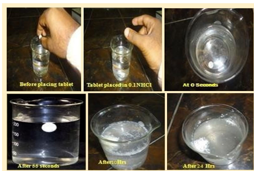
Fig 3: Photographs of formulation F10 during in vitro buoyancy study in 200 mL of 0.1 N HCl at different time intervals
