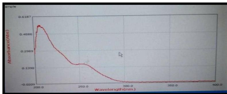
Figure 1: UV- spectrum of Sitagliptin phosphate pH 6.8
