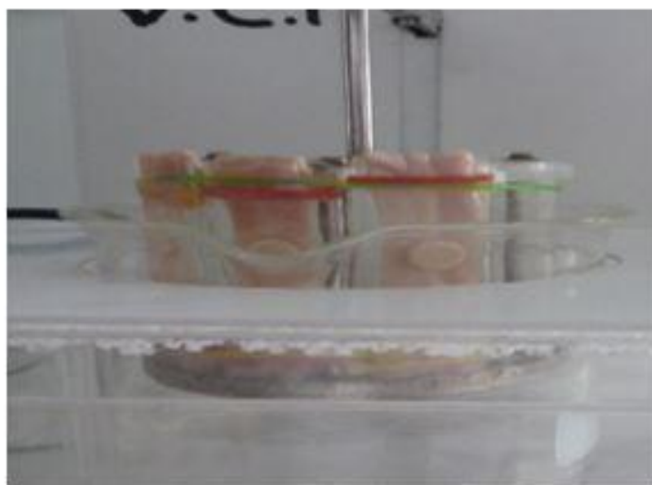
Fig: 10 Ex-Vivo Mucoadhesion test of Lafutidine mucoadhesive tablet
