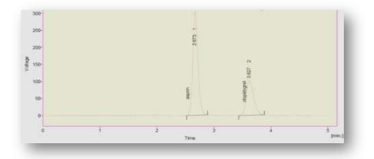
Figure 3: A Representative Chromatogram of Aspirin and Clopidogrel (Standard)
