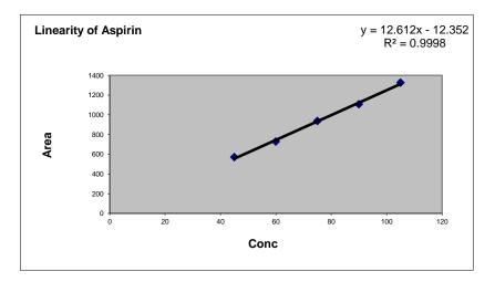
Figure 4: Linearity plot of Aspirin
