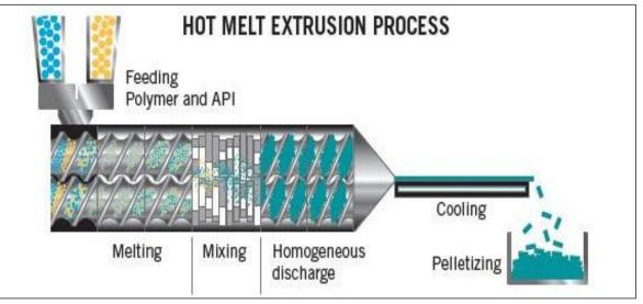
Figure 1: Schematic diagram of the HME process
