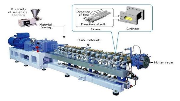
Figure 3: Twin Screw Extruder
